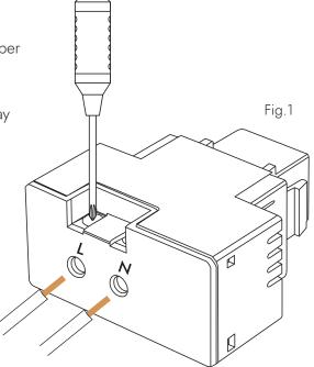
L – screw clamps for the phase wire N – screw clamps for
