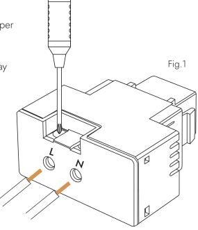
L – screw clamps for the phase wire
